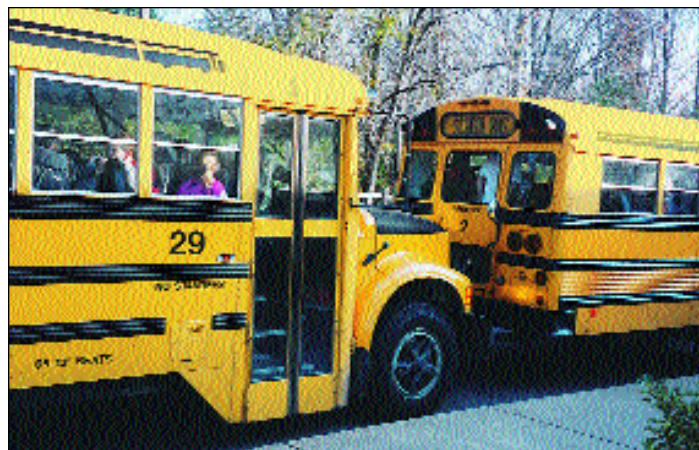
Queued Buses: Proximity of Doors to Tailpipes
